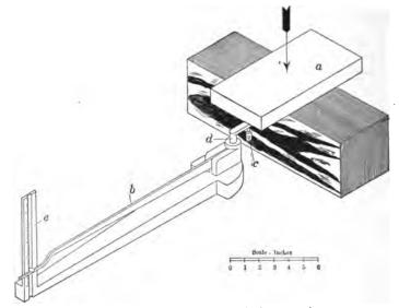
Fig. 6.—Compression perpendicular to grain.
